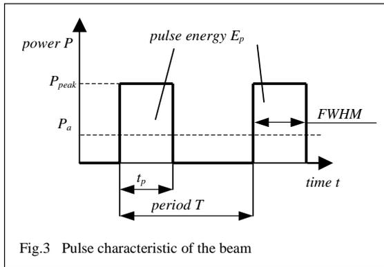
$P_a$  is the average power of the laser and  $t_p$  the pulse duration, which is practically defined by the FWHM (full width at half-maximum)
