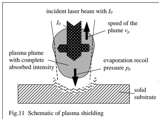
To reduce the influence of the LSDW one needs to dissipate the wave as fast as possible. One possibility in the practical design is the use of a focus lens with a short focus length (but  $z_r$  decreases too, see Eq.11).
