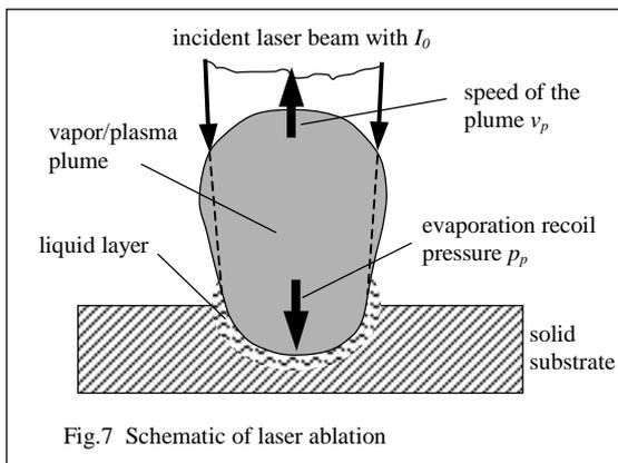
Fig.7 Schematic of laser ablation
