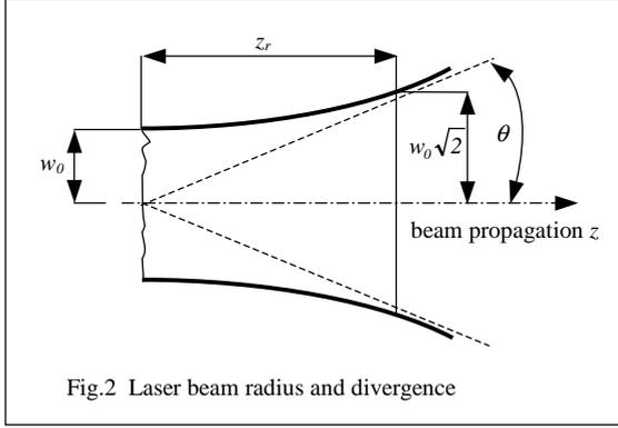
$M^2$  describes the beam quality and is called the **beam propagation factor** with an ideal theoretical value of  $M^2=1$  (TEM<sub>00</sub>-mode). In practical cases  $M^2$  lies between 1.2 and 15. Typical values of  $2 \cdot \theta$  are in the range of 1.1 ... 2.5 mrad ( $\approx 0.06 \dots 0.14^\circ$ ).
