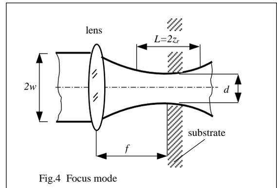
On condition that the divergence  $\theta$  of the input beam is small the diameter  $d$  within the focal plane of the lens can be approximately calculated by
